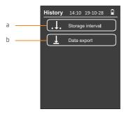
**Operation:** Press  $\blacktriangle$  or  $\checkmark$  to switch between **Storage interval** and **Data export**, then press  $\overset{\text{ok}}{\cup}$  to enter the corresponding interface.
