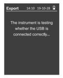
If connected to the computer successfully by the USB cable, the detector will pop up a tip **USB connection successful**; If not, it will remind you of the failure (See the figures below).
