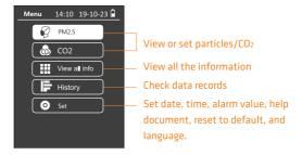
Note: It takes about 3 minutes for the CO<sub>2</sub> sensor to warm up and then enter detection status.
